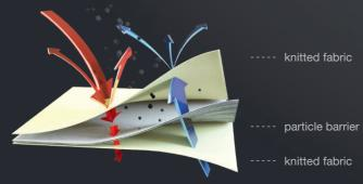
The material composition PP 3ly is made up of three layer knitted fabric, particle barrier, knitted fabric.
