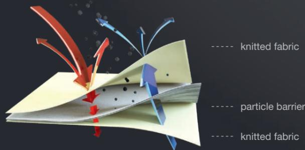
The material composition PP 3ly is made up of three layers: knitted fabric, particle barrier, knitted fabric.
